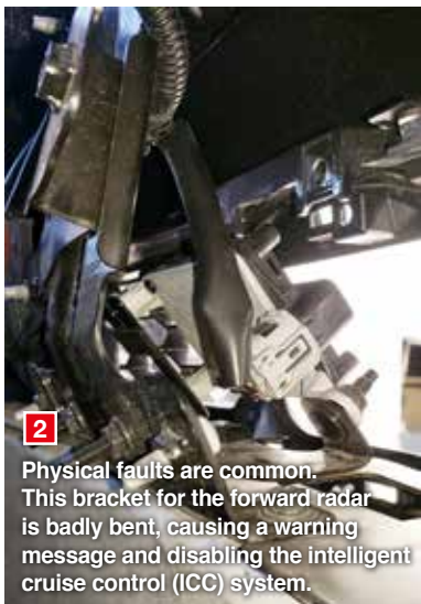
3 The bracket was bent back for diagnostic purposes. Proper repair required a new bracket and recalibration of the radar using specific targets.
