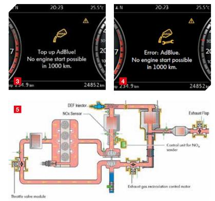
system occur between 220°C and 350°C, having just one injector and SCR catalyst at one point in the exhaust does not always give the optimum position for different engine loads.
