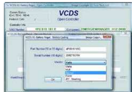
3 Ross Tech battery coding: Although physically capable, many Australian-sold batteries are not available for selection when coding in a new battery.
